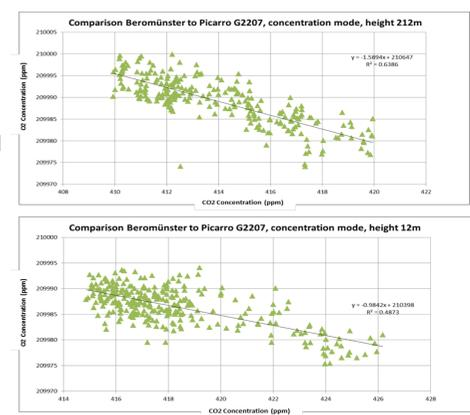
Figure 8. CO<sub>2</sub> and O<sub>2</sub> correlations at 12 and 212 m.
