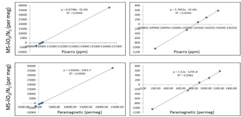
Figure 6. Measurement Correlation: MS vs Picarro and MS vs Paramagnetic
