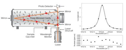
Figure 2. Schematic CRDS cavity and absorption spectrum.
