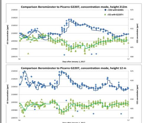
Figure 7. CO<sub>2</sub> and O<sub>2</sub> measurements at 12 and 212 m.
