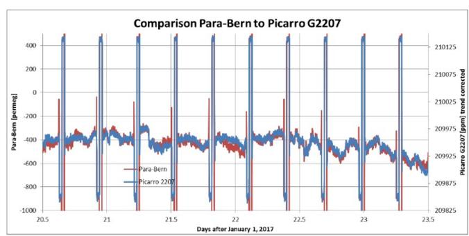
Figure 5. Calibrated dried outside air measurements from Picarro and Paramagnetic cell analyzer.
